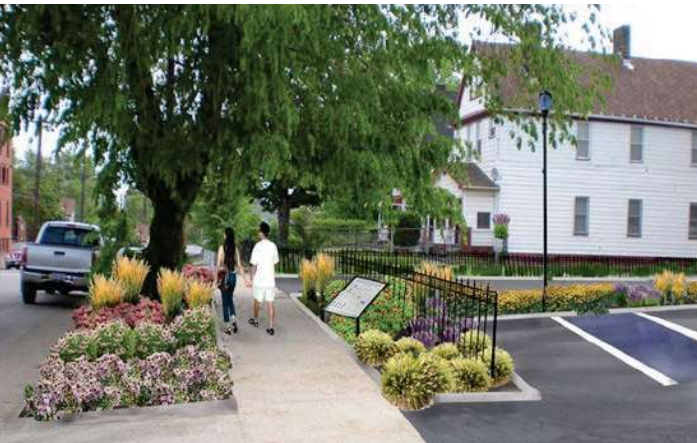
Parking lot in Tremont neighborhood designed by URS Corp. to provide bio-retention areas for managing stormwater; Illustration by: Katherine Holmok, URS Corporation
